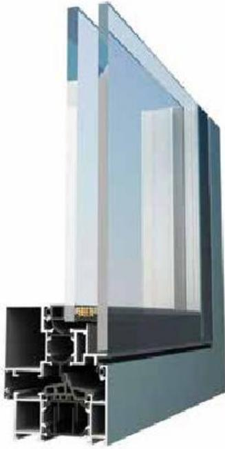
ICON 80 is a high performance system for windows & doors with its 70 mm frame depth, 34 mm glass fiber reinforced polyamide thermal-break and 3 compartmental structure.
