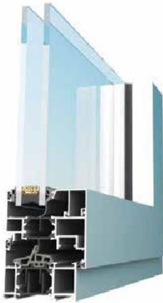
ICON 70 is a high performance system for windows & doors with its 70mm frame depth, 34 mm glass fiber re-enforced polyamide thermal-break and 3 compartmental structure.
