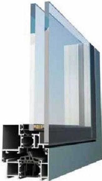
ICON 70 BV system enables transparent sash view from outside by bonding the glass to the sash. It is a highperformance economic alternative system for hidden sash windows with its 70 mm frame depth.
