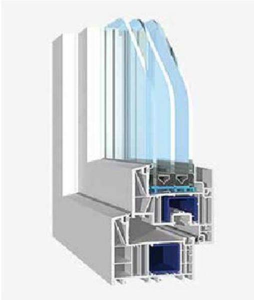
The innovative -6chamber design with a construction depth of 82 mm and sophisticated sealing technology ensures optimal thermal insulation and maximum energy efficiency.
